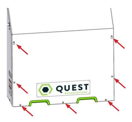
Replace access panel using T25 Torx driver to secure 7 screws.
