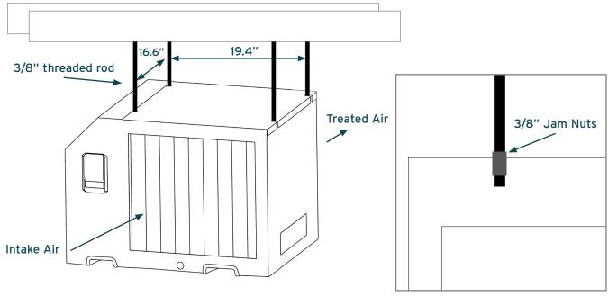
Parts Needed: 4 pieces - 3/8" threaded rod (not included) 4 pieces - 3/8" threaded jam nuts (not included)
