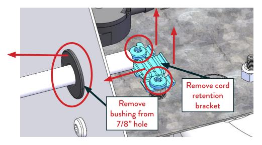
Remove the 2 screws holding the cord retention bracket using T25 Torx driver and remove retention bracket.
