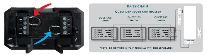
Red Arrow (top):Float jumper wire MUST stay in place or unit will go into error.Blue Arrow (bottom):This is an extra jumper wire that has no function in its factory-installed location.<br/>Move the wire up one spot to FAN and 24V for continuous fan operation.
