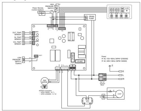
Figure 8 - Circuit Wiring Diagram
